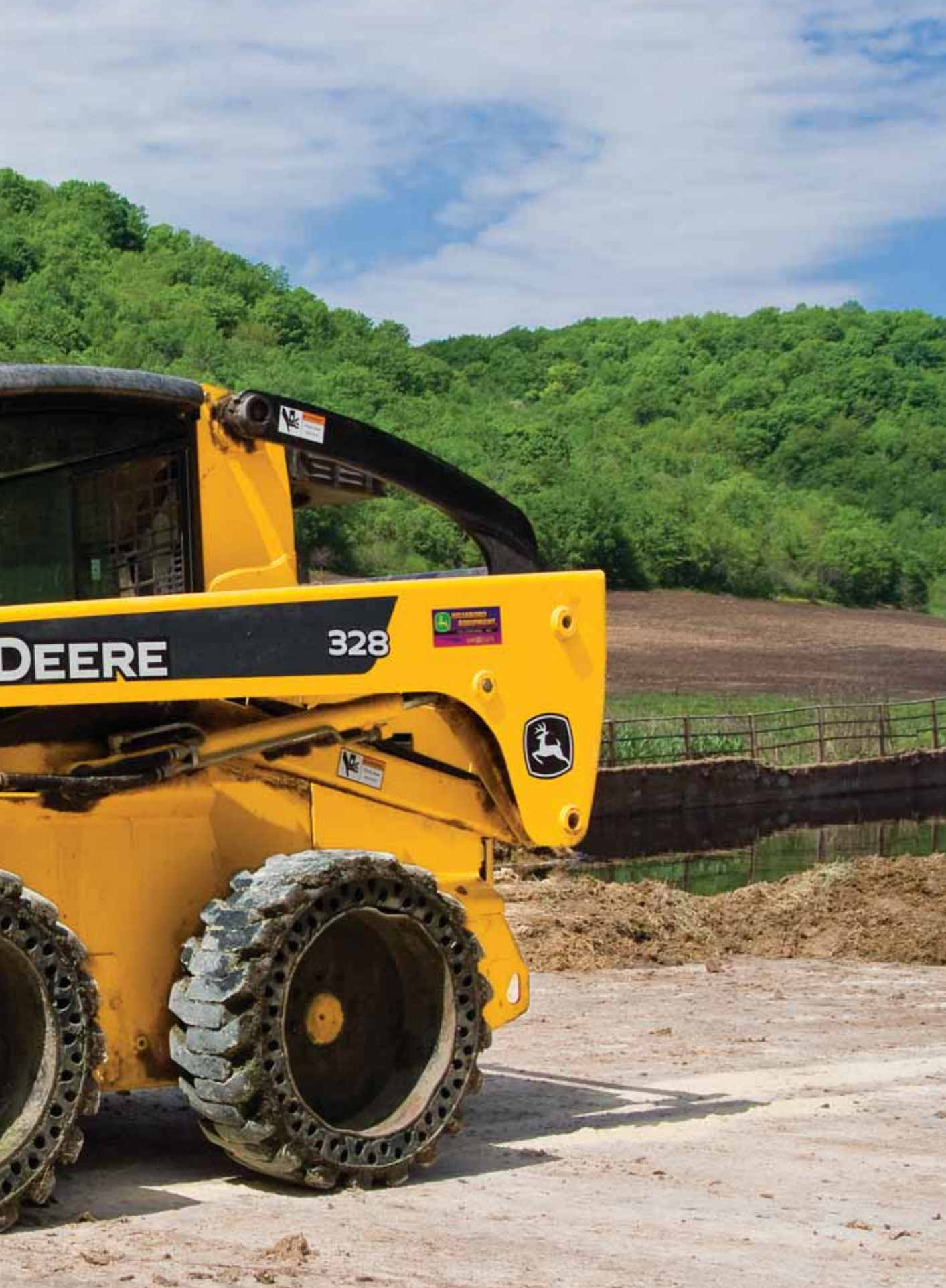
Tireless tire. Green Farms runs a solid flex tire manufactured by John Deere. "Flats are almost nonexistent," says Tom Green.
